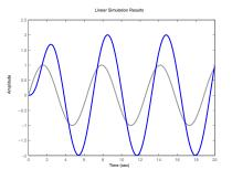
Frequency Response to  $\sin \omega t$  is given by  $G(\imath \omega)$
