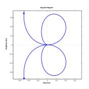
A plot of  $Re(G(\imath\omega))$  vs.  $Im(G(\imath\omega))$  as a function of  $\omega$ .
