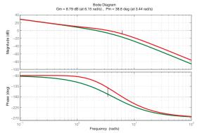
New Phase margin is  $38.6^{\circ}$ . New  $\omega_c = 4.79$ , new  $\omega_{BW} = 9$ .
