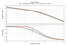
New Phase margin is  $65^{\circ}$ . New  $\omega_c=2.13$ , new  $\omega_{BW}=4$ .
