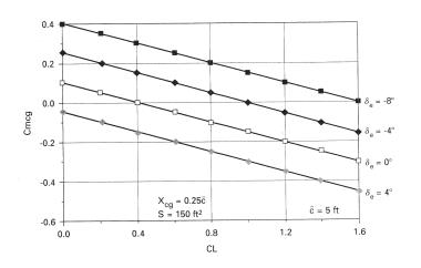
To trim for a flight condition, determine the required  $C_L$ . Then adjust  $\delta_e$  until  $C_M=0$  at  $C_{L.desired}$ .
