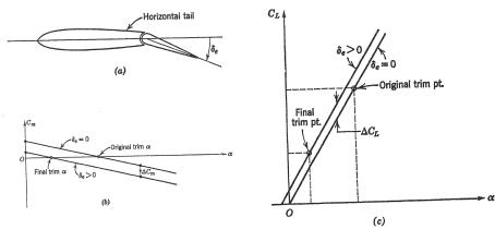
An elevator deflection changes the lift produced by the tail -  $C_{L0,t}$
