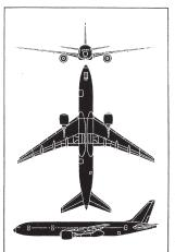
Notes: The latest airliner from Boeing, the 777 is also their first fly-by-wire. The outer 21 ft 3 in (6.5 m) of each wing can be folded upwards to reduce width at airport gates. The launch customer, United Airlines, took delivery of the first 777 in mid-1995.
