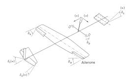
Control Surfaces on the **Wing** are called **Ailerons**
