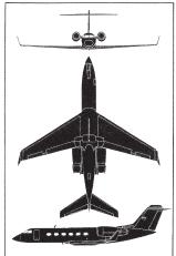
Notes: C-20 used by US armed services and Swedish Air Force (Tp 102). SRA-4s can be fitted with ventral canoe housing ECM, ESM, comms intercept or SLAR. Gulfstream IIs have no winglets, although many refitted with III wing.
