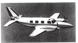
Dimensions: Length: 32 ft 7 in (9.9 m) Wingspan: 40 ft 8 in (12.4 m) Height: 13 ft (3.9 m)
