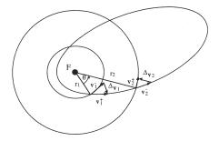
**Step 4:** Calculate  $\vec{v}_{tr,2}$  at the point of intersection with target orbit.
