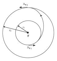
The Hohmann transfer is also the Maximum Time 2-impulse Transfer.
